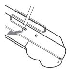
Attaching the supplied accessory to the handheld microphone (UTX-H1)
